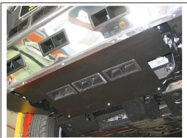
Figure 17: Centre under body guard fitted.
