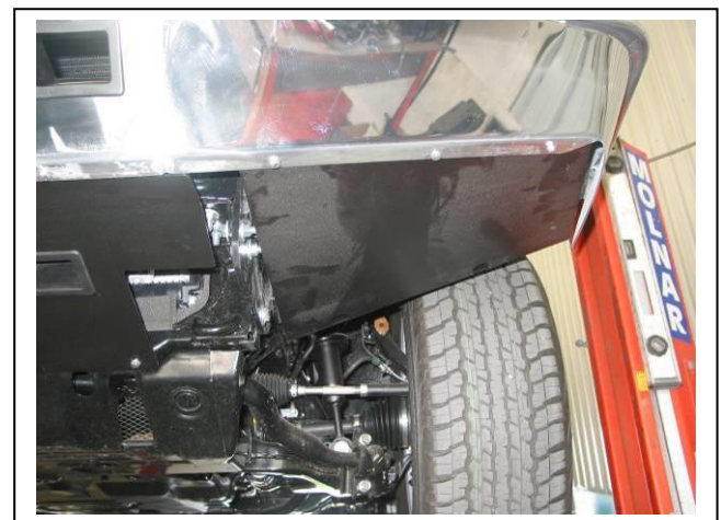
Figure 16: Passengers side under body guard
